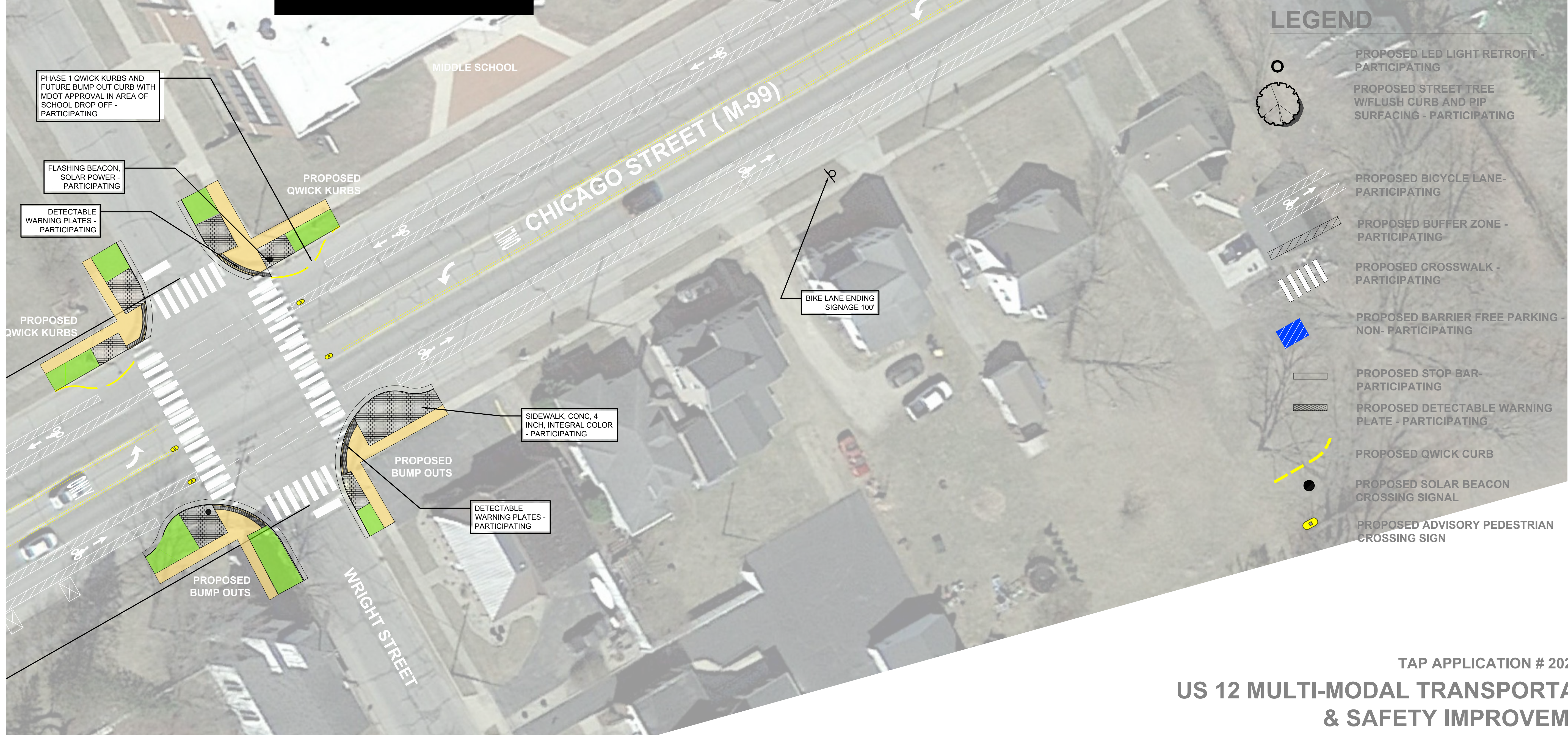
PHASE 1 - INSTALLATION OF QUICK KURBS AT MIDDLE SCHOOL NORTH SIDE CROSSING ON US-12. PHASE 2 WOULD INSTALL PERMANENT CURB WITH MDOT APPROVAL AFTER TRIAL PERIOD.
